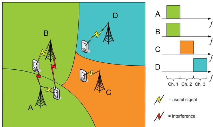
Figure 1: Neighbouring systems simultaneously using the same frequency can interfere with each other.
