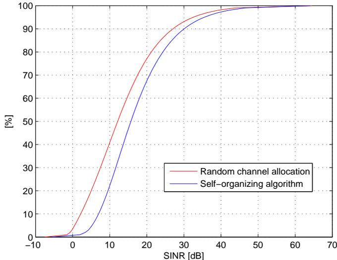
Figure 10: Comparison between random frequency allocation and proposed algorithm for the more realistic scenario.
