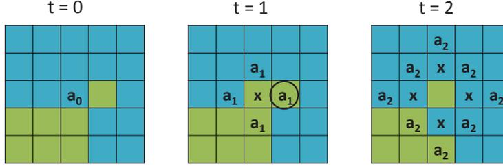
Figure 4: Von Neumann neighbourhood case. Green and blue are the only two colours, i.e. channels, available. We denote with  $X$  cells that changed their state in the previous time slot;  $a_t$  denotes cells which are active at time  $t$ . The decision of the cell circled in figure only depends on the interference resulting from the activity of cell  $X$ . Hence, this cell will select the blue channel even if the majority of its neighbours are using the same frequency.
