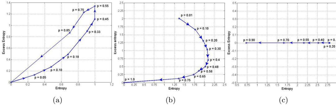
Figure 9: Complexity-entropy trajectory parameterized over the percentage  $p$  of inactive cells for: (a) regular channel assignment; (b) channel assignment resulting from the self-organising algorithm described in Section ; (c) random channel assignment.
