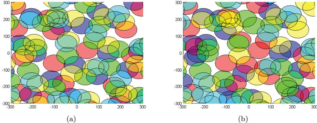
Figure 11: (a) Channel assignment resulting from the self-organising algorithm described in Section ,  $E_C = 0.55$  and  $h = 2$ . (b) Random channel assignment,  $E_C = 0$  and  $h = 2.32$ .
