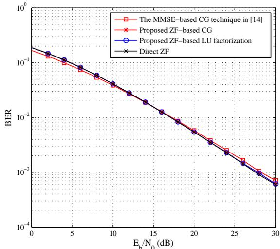
Fig. 11. BER performance of our proposed techniques compared with the direct ZF solution and the solution in [14] for the uplink of OFDMA systems with G-CAS, 4-QAM,  $N = 512$  and  $K = 4$  when  $|\epsilon_i| < 0.5$ .
