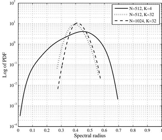
Fig. 6. Spectral radius of the matrix  $\mathbf{D}^{-1}\tilde{\mathbf{A}}$  for a system with the CFOs in the range of  $[-0.25, 0.25]$ .
