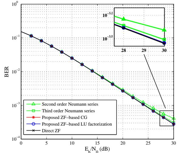
Fig. 9. BER performance of our proposed techniques compared with the direct ZF solution for the uplink of OFDMA systems with G-CAS, 4-QAM,  $N = 512$  and  $K = 4$  when  $|\epsilon_i| \leq 0.25$ .
