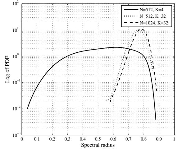
Fig. 7. Spectral radius of the matrix  $\mathbf{D}_P^{-1} \tilde{\mathbf{P}}$  for a system with the CFOs in the range of  $[-0.25, 0.25]$ .
