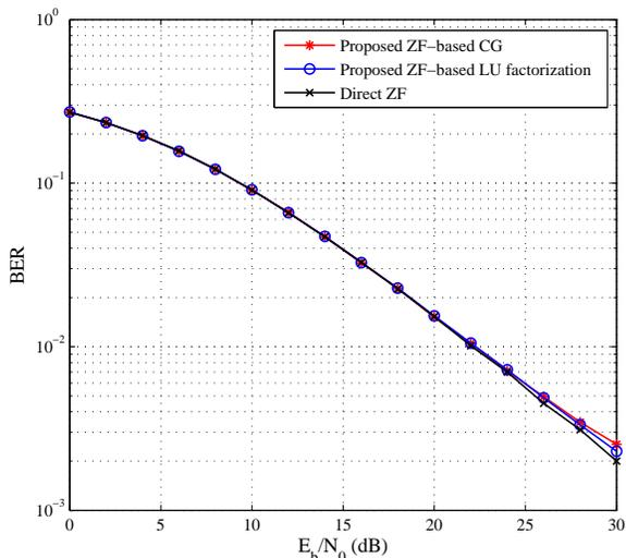
Fig. 12. BER performance of our proposed techniques compared with the direct ZF solution for the uplink of OFDMA systems with G-CAS, 16-QAM,  $N = 1024$  and  $K = 32$  when  $|\epsilon_i| < 0.5$ .
