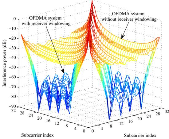
Fig. 2. Interference power between different subcarriers for G-CAS case when  $N = 32$ ,  $K = 4$ ,  $N_w = 8$ , CFOs =  $[0.20, -0.35, 0.45, -0.11]$  for the systems with and without receiver filtering.
