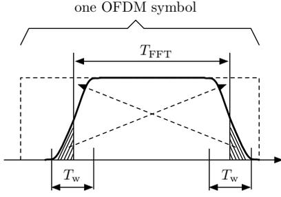
Fig. 1. A raised-cosine window and the process of aliasing in time domain. The excess samples beyond the length  $T_{\text{FFT}}$  on each side are added to the attenuated samples on the other side.
