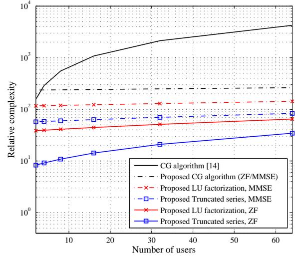
Fig. 8. Relative complexity of different CFO compensation techniques with respect to single user case when  $N = 2048$ .
