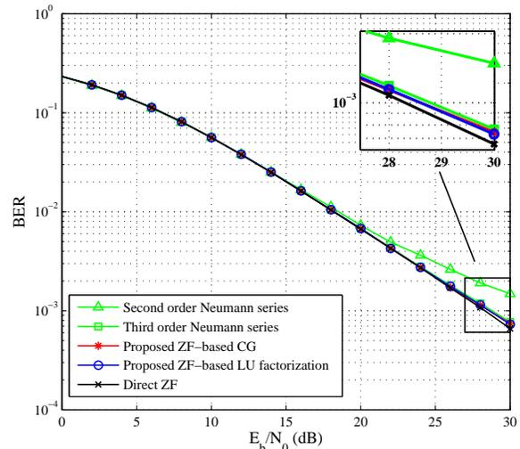
Fig. 10. BER performance of our proposed techniques compared with the direct ZF solution for the uplink of OFDMA systems with G-CAS, 16-QAM,  $N = 1024$  and  $K = 32$  when  $|\epsilon_i| \leq 0.25$ .
