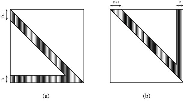
Fig. 4. (a) and (b) depict the structure of  $\mathbf{L}$  and  $\mathbf{U}$  matrices after LU factorization of a quasi-banded matrix, respectively.
