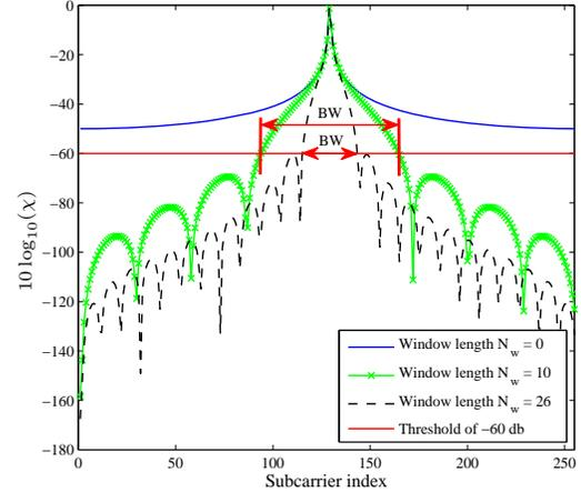
Fig. 3. Interference power for different values of  $N_w$  and the threshold line of -60 dB for an uplink scenario where  $N = 256$  and  $\epsilon_{\max} = 0.4$ .
